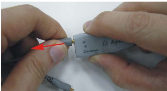
Figure 3-1 Pull the probe head straight out to disconnect it from the amplifier.
