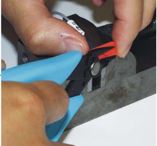
Figure 3-12 Cut the wires even with the trim gauge
